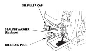
4. With the engine in a level position, fill with the recommended oil to the upper limit of the oil filler neck (see page 34).
