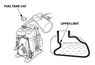
After refueling, reinstall the fuel tank cap securely.
