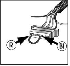
Testing the actual output of the alternator is known as "Full Field Testing". This can be accomplished by jumping a positive 12VDC current to the field terminal at the rear of the alternator. This test eliminates both the regulator and the harness, making it easier to isolate your investigation to the alternator.
