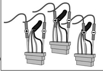
PLEASE NOTE: In systems where the ignition (BROWN) wire is supplied power via an oil pressure switch, jump directly from test #1 to test #3.
